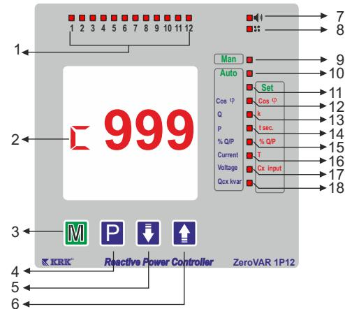
**1- 1.2.3.....12:** Shows the steps which capacitor is switched on.
