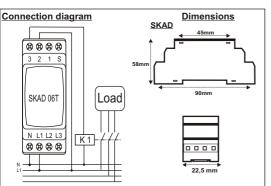
If phase sequence control is not desired "S" - "N" must be short-cut.
