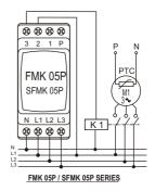
NOTE: fmk 05P / sfmk 05 P series P and N to cancel the PTC protection Short circuit ends.
